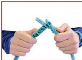
1. Holding the belt with the tabs upwards, let the tab of one belt's end get through two links at once. (three if C section)
